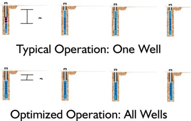
Figure 3. Utilizing simple math in SCADA, the drawdown of wellfields is optimized to minimize pumping costs.
